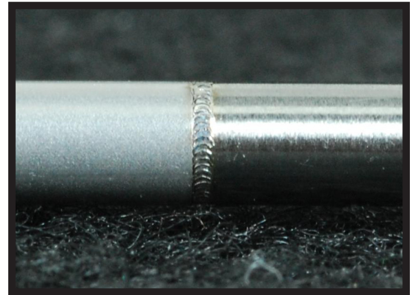
Nitinol welded to 316 stainless steel tube Outside diameter: 0.095"
