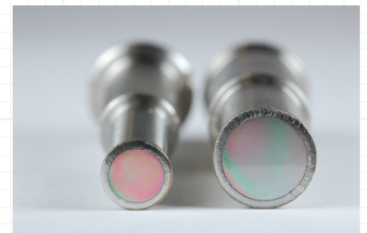
Tube Weld = 304 Stainless Steel
